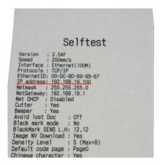
Note: if the above methods to modify the IP address are not successful, it's suggested that the computer IP address and the printer IP address shall be set within the same network segment: 192.168.123. XXX, before connecting the printer (excluding the router method) to the computer and using tools to modify the IP. Specific method is as follows:
