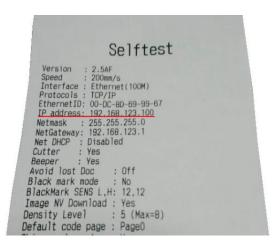
2. Confirm the printer IP address and then connect the printer to a computer through a hub, switch or cable directly (direct interconnection method). (Note: the IP address may not be modified if the connection is established through a router) Change the IP address by the test tool software in the CD, the software is as follows:
