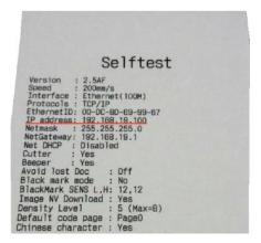
The above self test page shows that the new IP address has been set successfully. This method is suitable for all Ethernet port printers.
