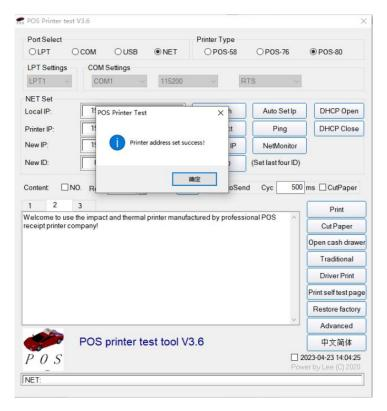
4. After the prompt window indicating "printer address successfully set" appears, print selftest page again to see if the IP address has been modified, as shown in the picture below:
